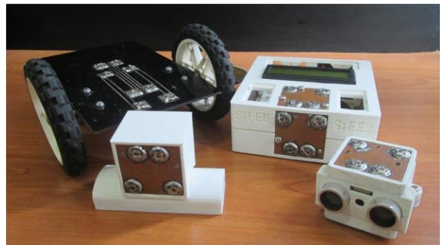
Figure 1. Disassembled modules of initial prototype.
