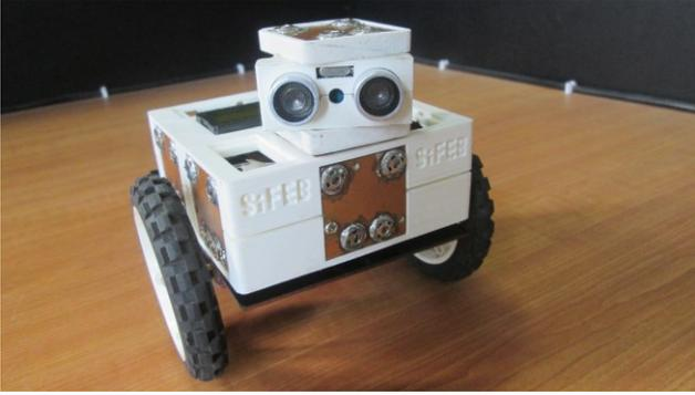
Figure 2. An obstacle avoiding robot using SiFEB's initial prototype.
